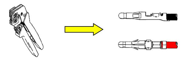
Pin Terminals are fitted to Molex Connector Housing as shown:
